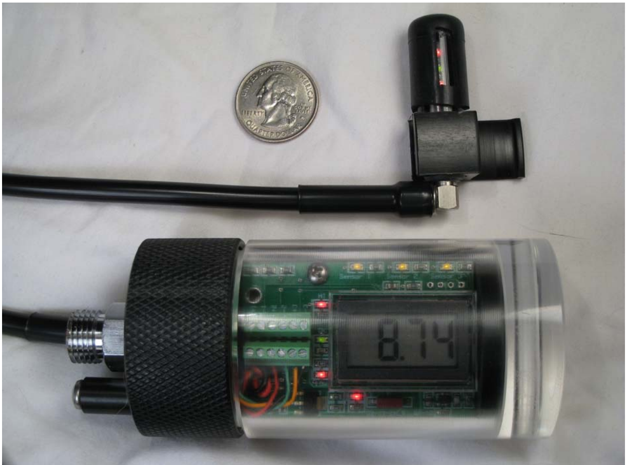
Assembled Left Side G2 PPO2 Monitor shown with optional HUD
